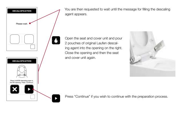
If you cancel the process, the boiler is flushed with fresh water. Once the suggested decalcification process is initiated, we recommend that the process is allowed to finish completely.
