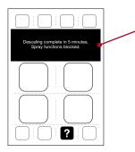
The decalcification program is started. The remaining process time is shown on the display.
