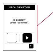
The remote control switches to the "Decalcification" menu. Start the process as described in section 10.11, Decalcification, automatic.
