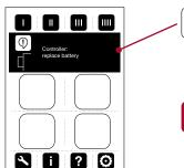
Message 2: "Controller: Replace battery" Your remote control indicates "Controller: Replace battery". Press "Service info" to view the instructions for replacing the battery.
