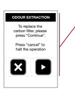
The remote control switches to the "Odour extraction" menu. Proceed as described in section 10.13, replacing the odour filter automatically.
