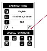
Thermal cleaning flushes the entire water-carrying system on your shower toilet with hot water to eliminate bacteria and germs. An illuminated red LED display on the appliance and corresponding service information on the remote control remind you when thermal cleaning is due. The automatic reminder is activated by default and can be deactivated by pressing "Thermal cleaning". The automatic reminder then no longer appears.
