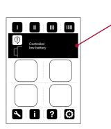
Message 1: "Controller: low battery" Your remote control indicates "Controller: low battery". Please purchase a 3-volt battery, type CR2032. Replace the battery after the second message appears.
