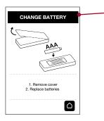
If only the instructions for replacing the battery appear on the remote control and the backlighting on the display is off, the batteries must be replaced immediately.
